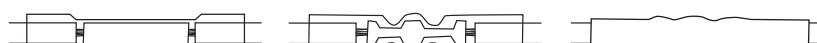
1. Strip wires 1/4" and insert into crimp barrel of connector. 2. Crimp the wires in crimp barrel. 3. Apply heat until tubing recovers and adhesive melts and flows.
